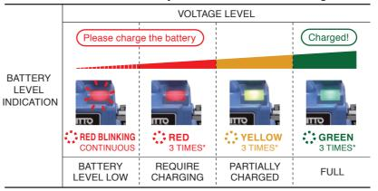
\*After the lamp flashes 3 times with the color according to the battery level, the lamp turns green
